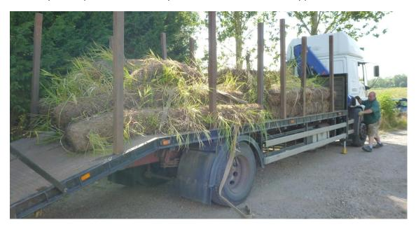
The reed plants are set in a 'sausage' shaped tube of coconut matting measuring 3 metres length and about 0.3 metres diameter all held together by netting mesh. We ordered 30 of these.
